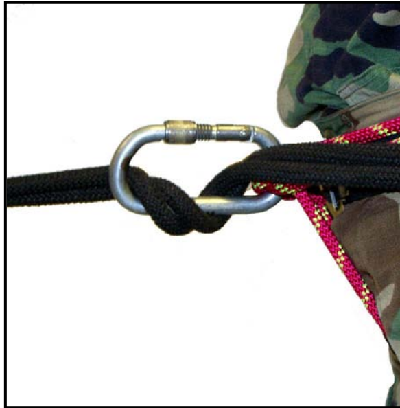
Figure 7-7. Proper hookup using carabiner wrap.
